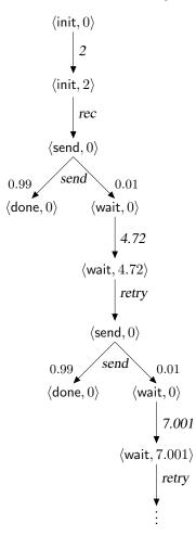
Figure 2. An example of behaviour for the simple communication protocol given in Figure 1.
