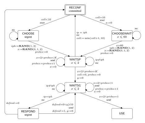
Figure 5. Probabilistic timed automaton for the concrete host (model Reset)
