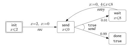
Figure 1. A probabilistic timed automaton modelling a simple communication protocol.
