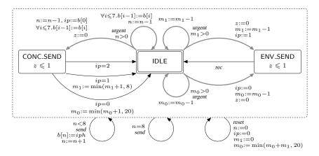
Figure 6. Probabilistic timed automaton for the environment (model Reset)
