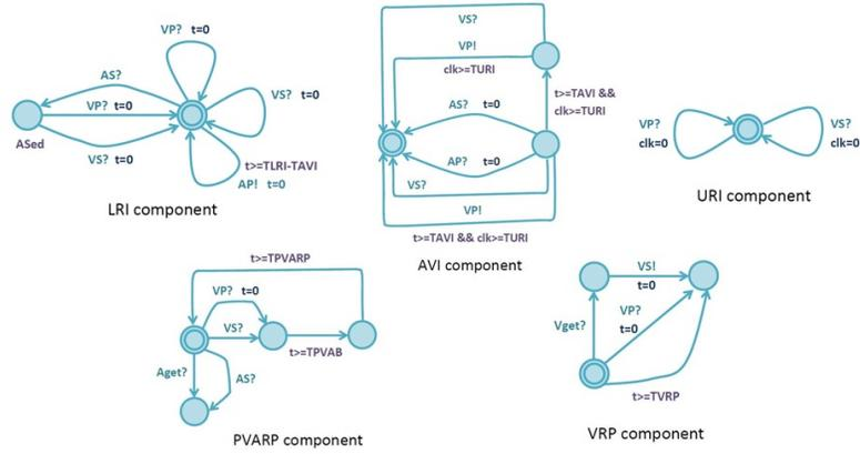
Figure 4: Timed automata as described by Jiang et al[7]
