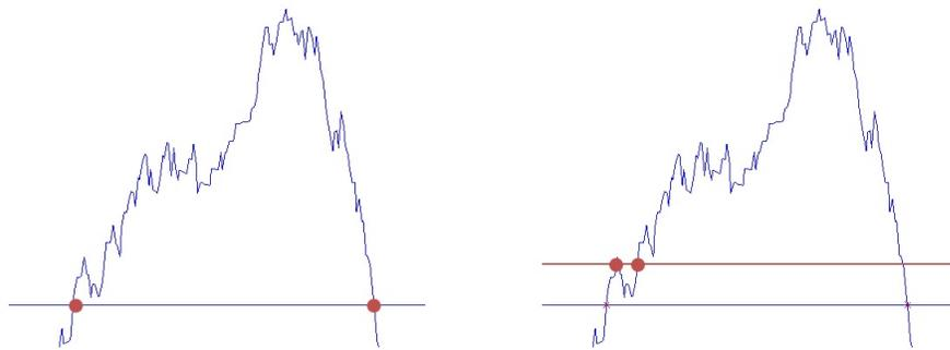
Figure 2: Gritzali method for defining wave duration
